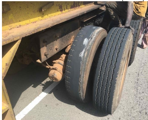
Figure 4.9 – Defective tyres in Liberia (Jan'18)
